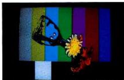
A low-gain RGB chroma nulled key places the flowers and vase over bars. With high gain, the flowers remain realistic, while the vase takes on a surrealistic aspect.
